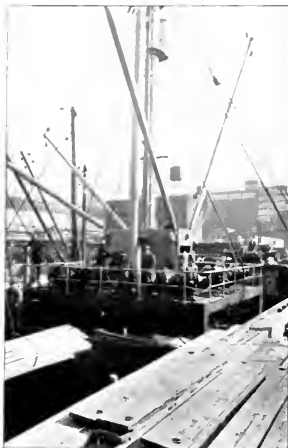
View on the American motorship Seekonk showing method of installing deck winches on platform which has been found ideal in vessels carrying deck loads.
